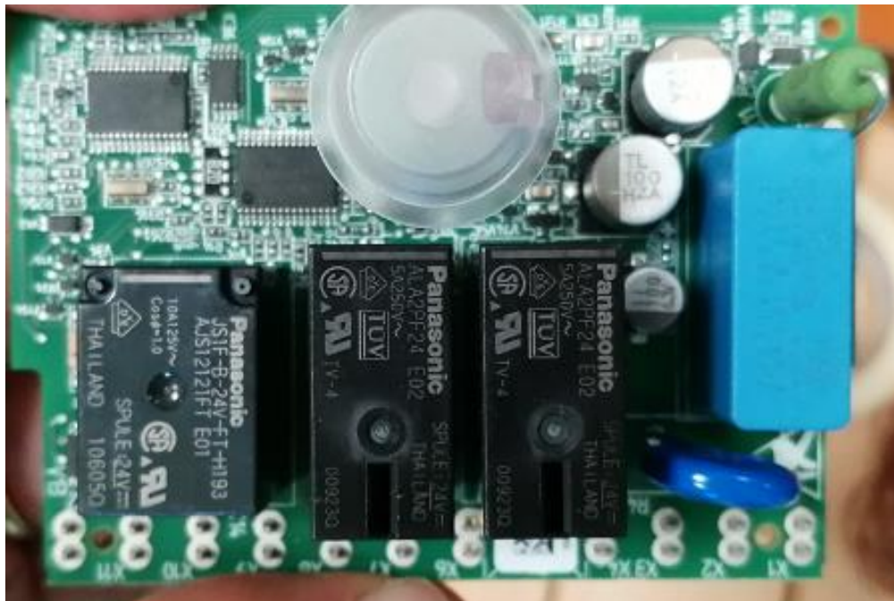
Ignition board unit PCB (front)
