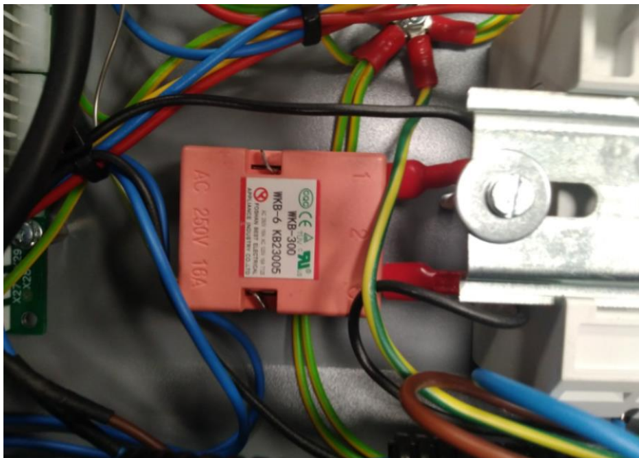
Capillary self resetting thermal cut-out
