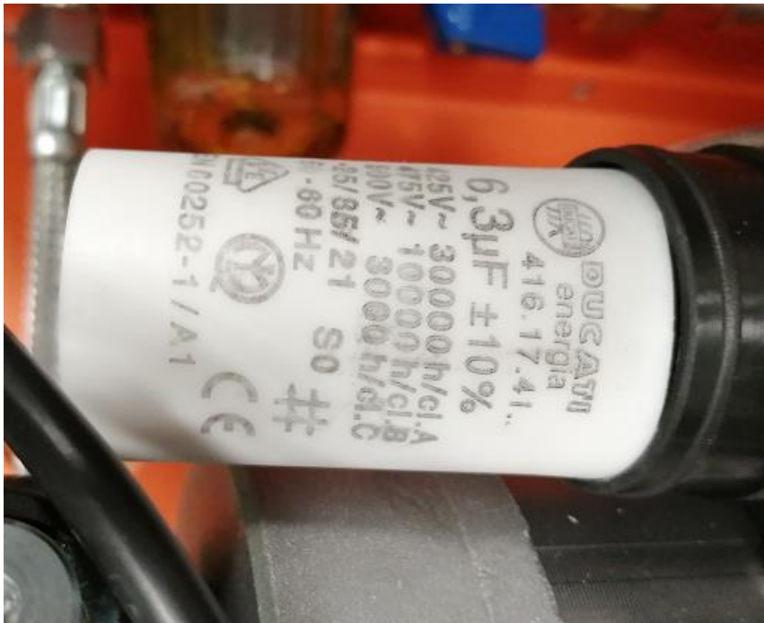
Oil pump motor capacitor
