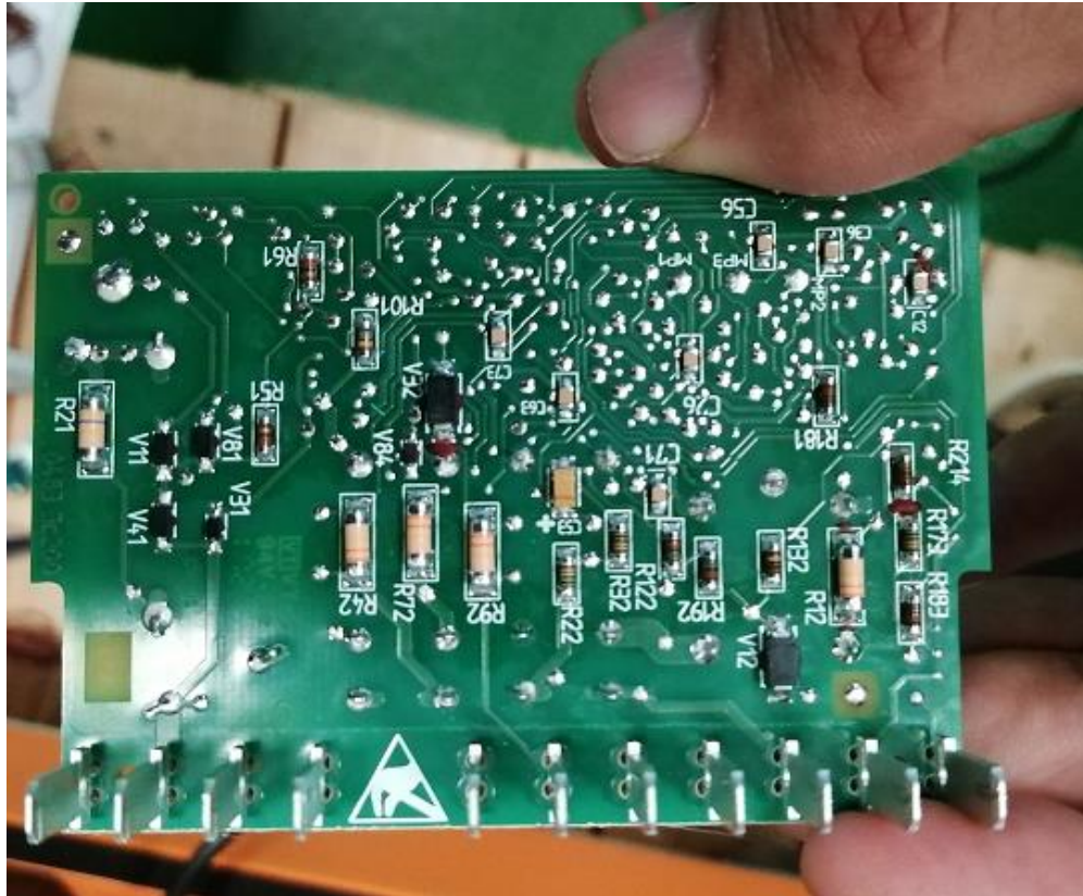
Ignition board unit PCB (rear)
